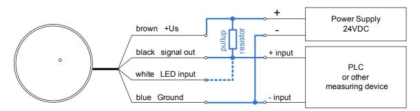
The connection is done based on the drawing above. The dashed line connects the LED drive input to the output, if you intend to indicate pulses on the meter itself.
