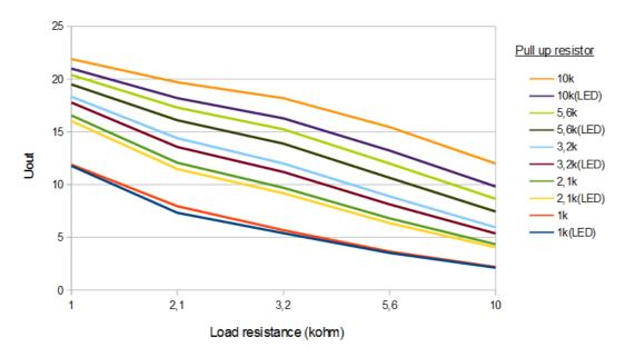
If you do not know the levels and the input resistance, use 2,2kohm pull-up resistor, that will work in most of the cases. If you select 1k pull-up resistor you must know that it can lead 24mA current in off state which is more than 0,5W dissipation!
