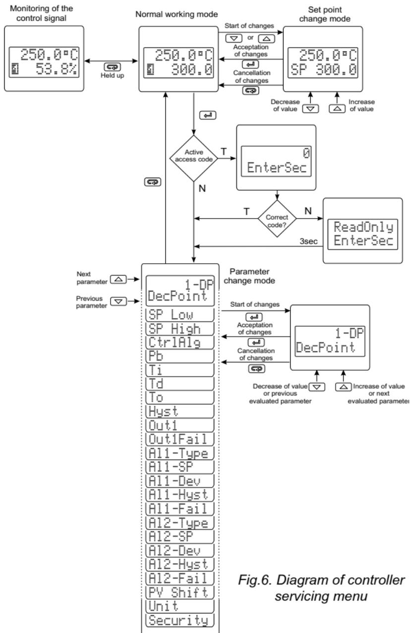
Fig.6. Diagram of controller servicing menu
