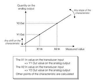
Fig. 6. Individual characteristic of analog outputs
