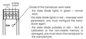
Fig. 3. View of the P20 transducer
