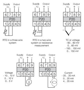
Fig.2. Electrical connection diagrams of the P20 transducer.
